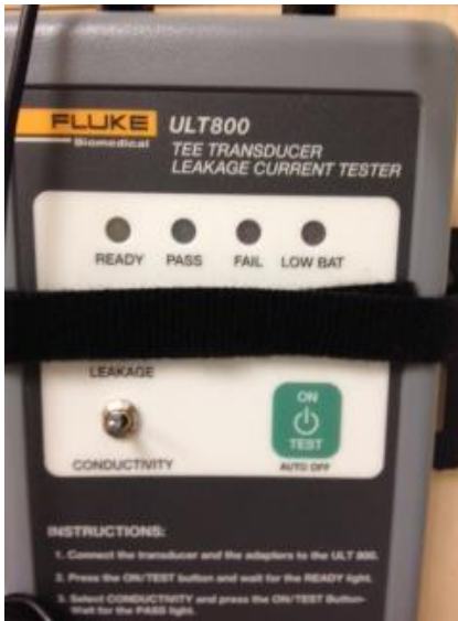
Leakage Current Tester Control Box
